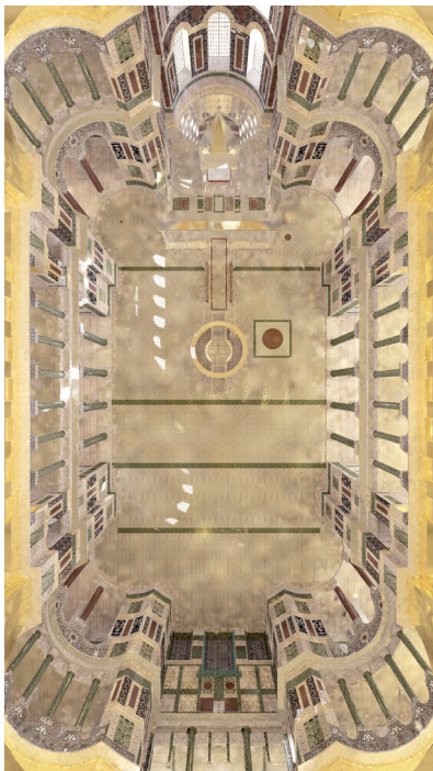
Fig. 5 Hagia Sophia, reconstruction of a view from above, revealing the organization of space under the dome (© Lars Grobe, Oliver Hauck, Martin Kim, Andreas Noback, Rudolf H.W. Stichel, Helge Svenshon, Technische Universität Darmstadt)
